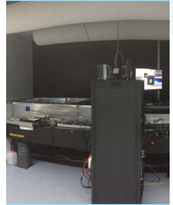
High Energy, High Power Few Cycle OPCPA prototype laser system. High-power pump source, based on regenerative thin-disc amplifier. Repetition rate 6 kHz
